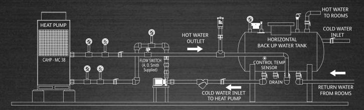
Storage tank: Minimum 2000 & 4000 litre for 5HP & 10HP respectively Circulation pump flow rate: 3500 LPH & 6500 LPH for 5HP & 10HP respectively
